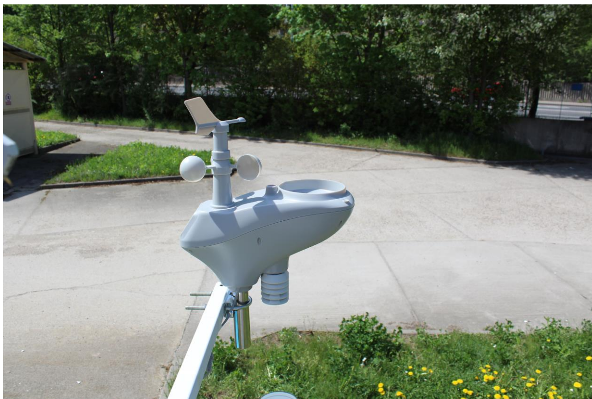
Detail Meteostanice Eurochron
